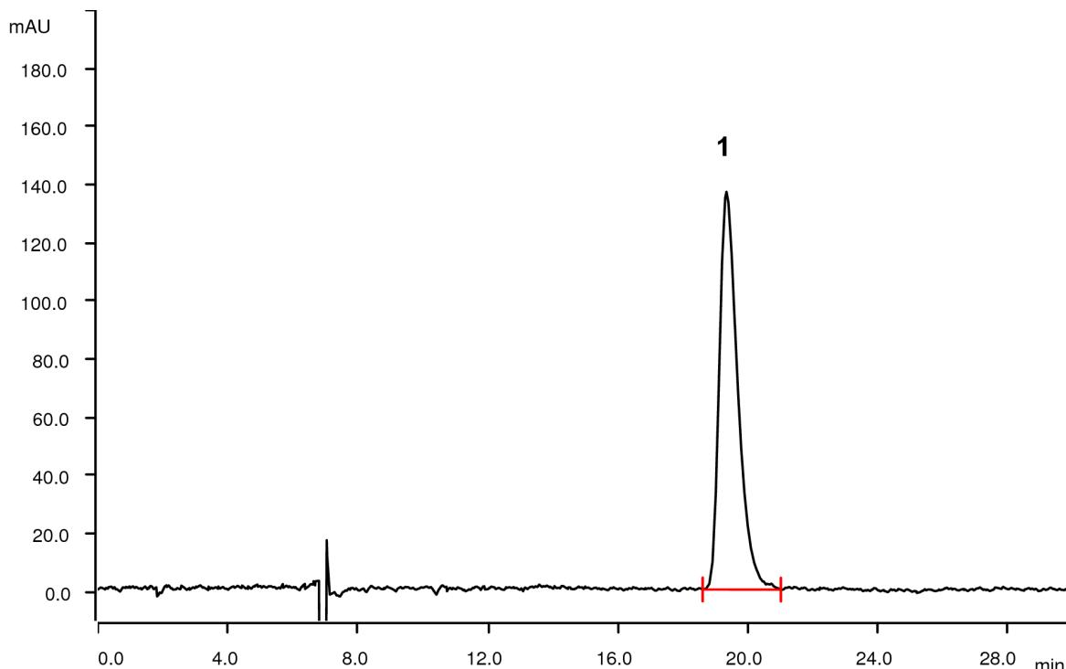
USP is updating the General Chapter <591> «Zinc Determination» monograph to include ion chromatography as a method for the assay. Zinc oxide is used in various skin care creams, drugs, and drug products. The ion chromatography analysis involves separation of zinc using, e.g., L91 (Metrosep A Supp 10) followed by post-column reaction using 4-(2-pyridylazo)resorcinol (PAR) reagent and subsequent detection at 530 nm wavelength.
